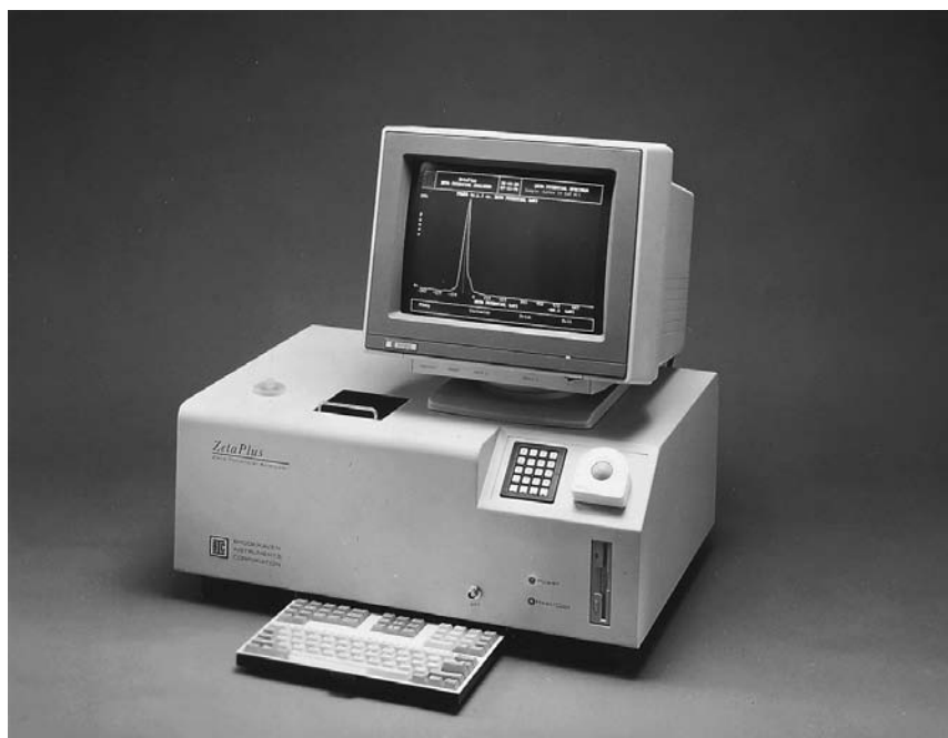
Plate 7.9 — Brookhaven's ZetaPlus PCS particle sizer which also can measure the zeta potential (courtesy Brookhaven Instruments Inc.).
